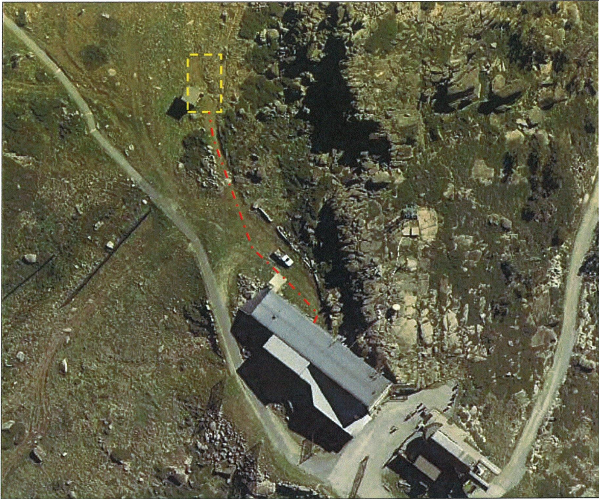
Figure 9: Diagram illustrating the proposed location of the components of the project (with the hut location illustrated in yellow and the services trench in red)
